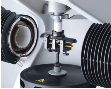
Figure 59. PCB sample installed in the 3-point bending accessory in the DMA/SDTA 1+.
