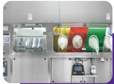
Energy efficient LED coloured lighting to provide quick visual feedback of current STIW status
