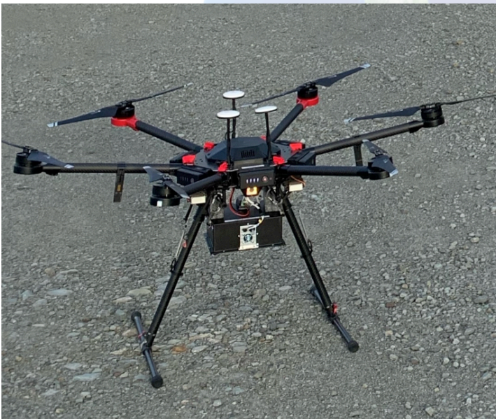
The compact, lightweight MIRA Strato is easily adapted to many commercially available drones (DJI Matrice 600 shown), and can be mounted in any orientation. Communication is typically achieved via the RS-232 port, which can stream at data rates of up to 10Hz. The Strato is inherently immune to vibrations, and has proven robust in many drone studies to date. (Photo courtesy of Scientific Aviation)
