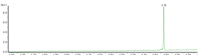
Figure 4: UPLC Chromatogram of Ac-ELLELDK(-A)WASLWN-NH 2 , synthesized via ivDde-deprotection.
